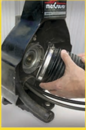
Mercruiser Gimbal Housing Repair
